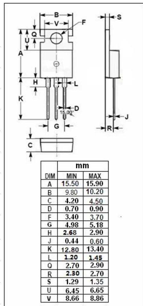
**isc N-Channel Mosfet Transistor****BUZ30A****ELECTRICAL CHARACTERISTICS****T<sub>c</sub>=25°C unless otherwise specified**
