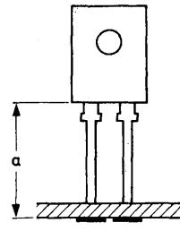
at a lead-length  $a = 3 \text{ mm}$
