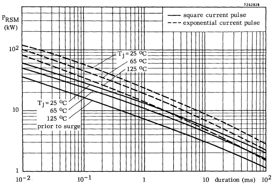
Duration of an exponential pulse is defined as the time taken for the pulse to fall to 37% of its initial value. It is assumed that the energy content does not continue beyond twice this time.
