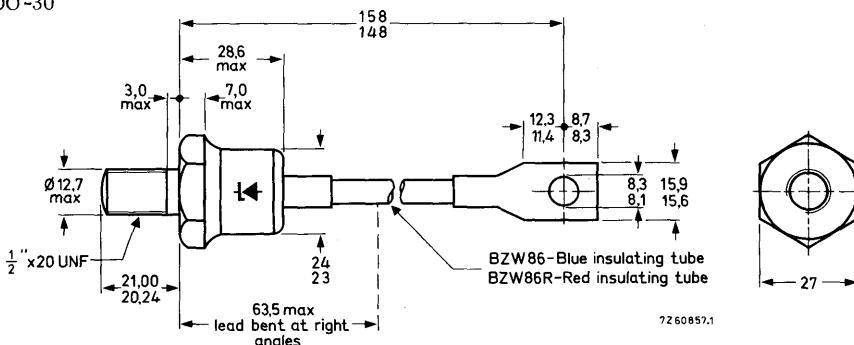
Supplied with device: 1 nut, 1 lock washer
