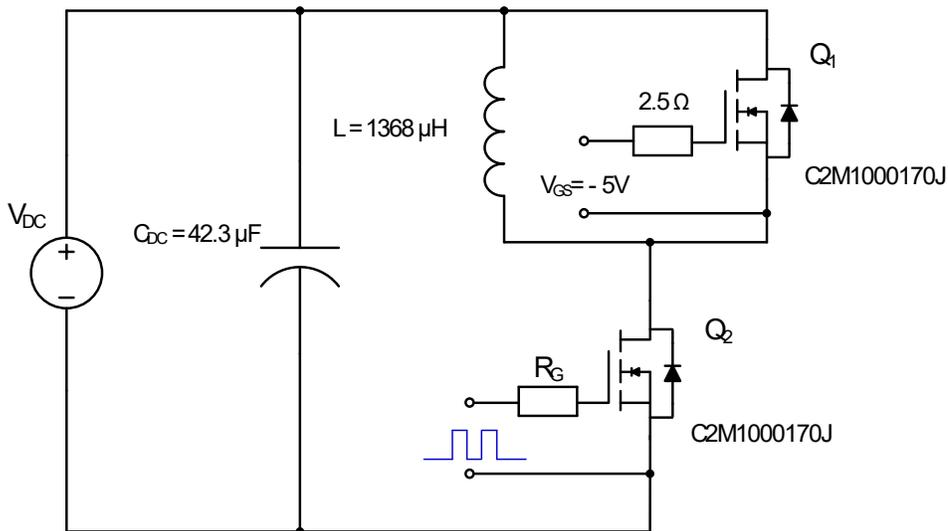
**Figure 29.** Clamped Inductive Switching Waveform Test Circuit
