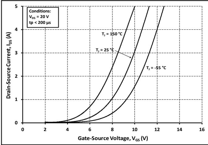
Figure 7. Transfer Characteristic for
