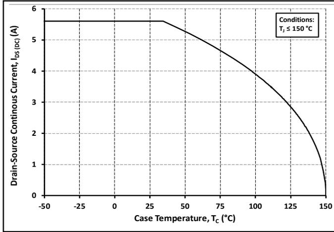
Figure 19. Continuous Drain Current Derating vs. Case Temperature
