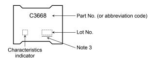
Note 3: A line under a Lot No. identifies the indication of product Labels. Not underlined: [[Pb]]/INCLUDES > MCV Underlined: [[G]]/RoHS COMPATIBLE or [[G]]/RoHS [[Pb]]
