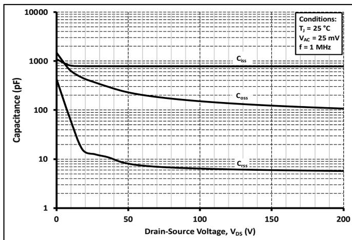
Figure 17. Capacitances vs Drain-Source Voltage (0 - 200 V)
