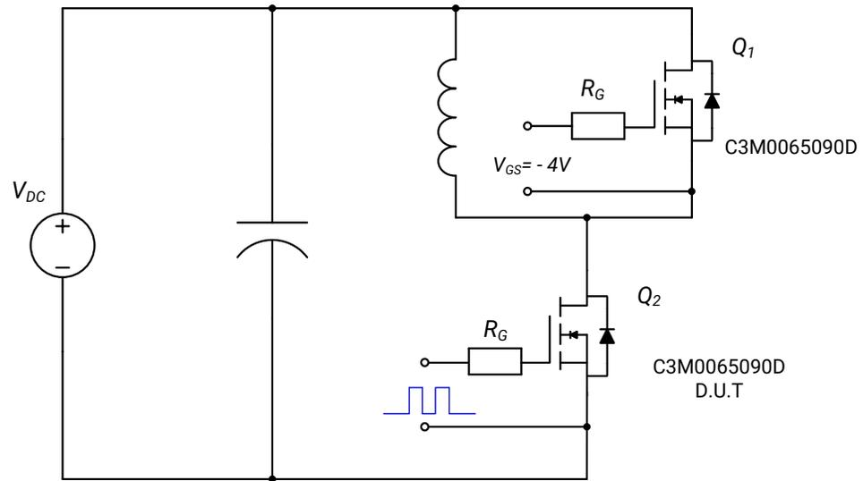
**Figure 30.** Clamped Inductive Switching
