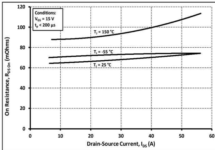
Figure 5. On-Resistance vs. Drain Current For Various Temperatures
