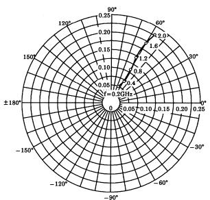
$\begin{array}{l} \text{S}_{22e} \\ \text{V}_{\text{CE}} = 5\text{V} \\ \text{I}_{\text{C}} = 5\text{mA} \\ \text{Ta} = 25^{\circ}\text{C} \\ \text{(UNIT}: \Omega) \end{array}$
