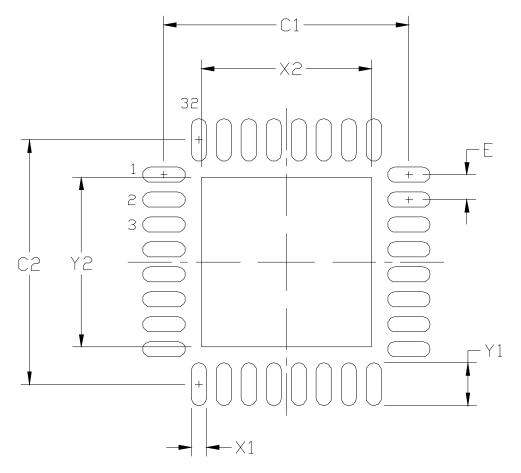
Figure 6.2. Typical QFN-32 Landing Diagram
