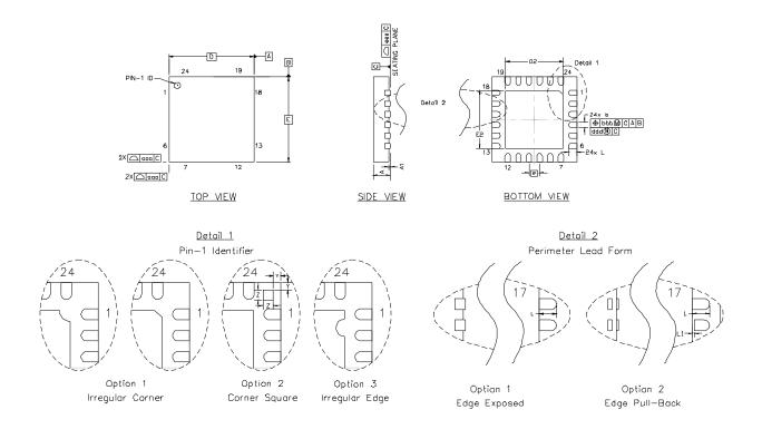
Figure 7.1. QFN-24 Package Drawing
