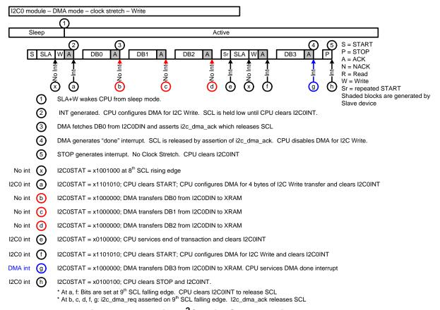
Figure 30.7. Typical I<sup>2</sup>C Write Sequence in DMA Mode
