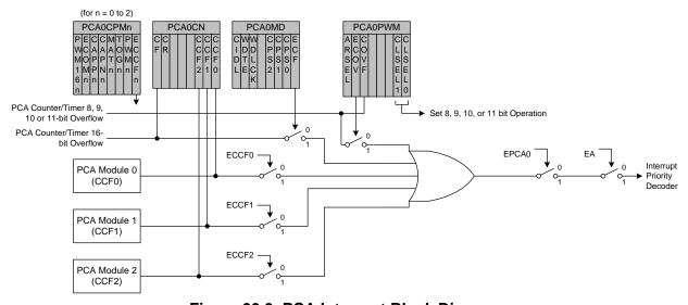
Figure 33.3. PCA Interrupt Block Diagram
