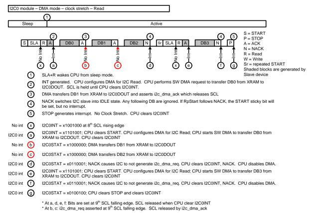
Figure 30.8. Typical I<sup>2</sup>C Read Sequence in DMA Mode
