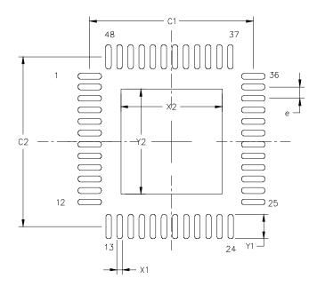
Figure 5.2. QFN-48 Landing Diagram
