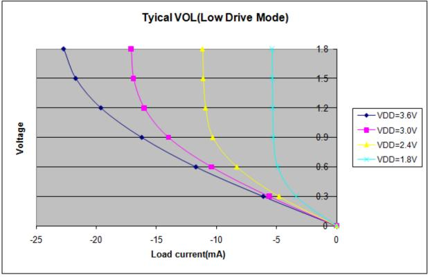
Figure 1.2. Typical VOL Curves, 1.8–3.6 V
