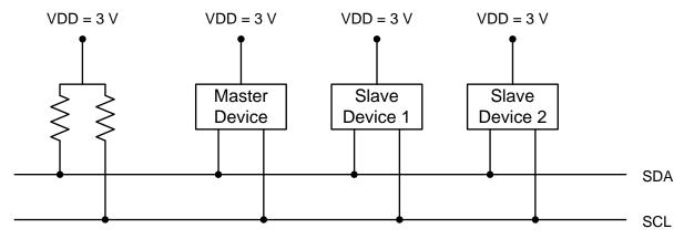
Figure 30.2. Typical I<sup>2</sup>C Configuration
