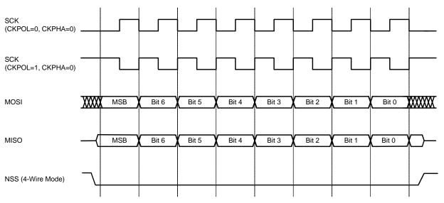
Figure 28.6. Slave Mode Data/Clock Timing (CKPHA = 0)
