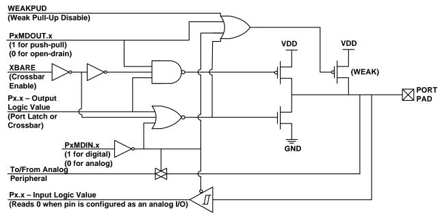
Figure 26.4. Port I/O Cell Block Diagram
