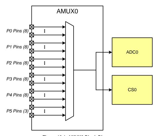
Figure 19.1. AMUX0 Block Diagram
