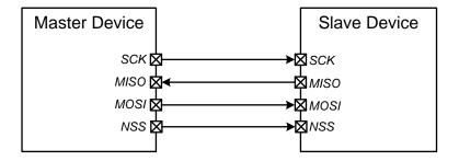
Figure 28.4. 4-Wire Single Master Mode and 4-Wire Slave Mode Connection Diagram
