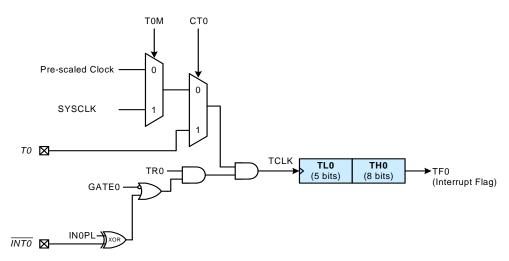
Figure 32.1. T0 Mode 0 Block Diagram
