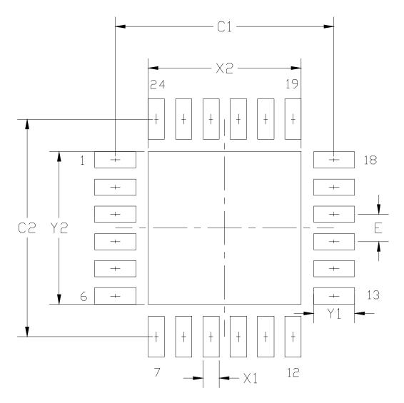
Figure 7.2. Typical QFN-24 Landing Diagram
