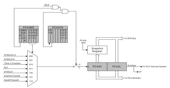
Figure 33.2. PCA Counter/Timer Block Diagram
