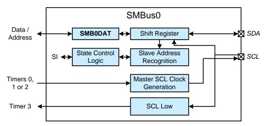
Figure 29.1. SMBus0 Block Diagram
