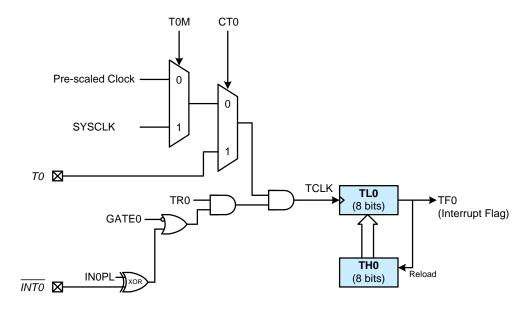
Figure 32.2. T0 Mode 2 Block Diagram
