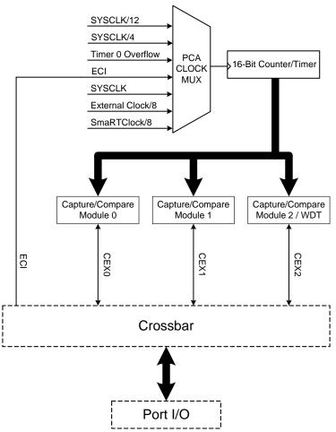
Figure 33.1. PCA Block Diagram
