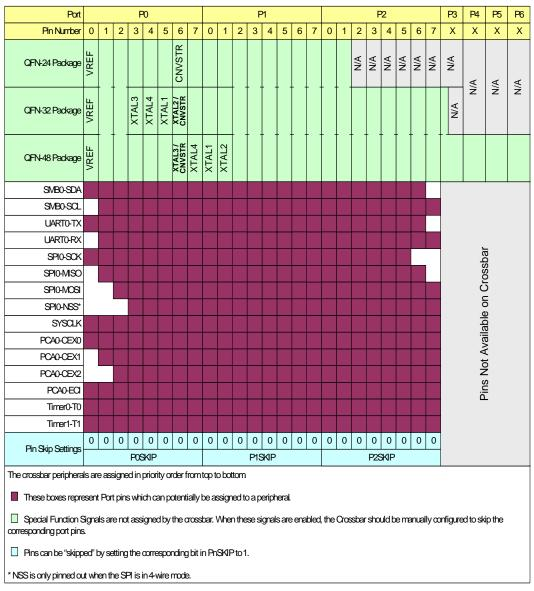
Figure 26.2. Crossbar Priority Decoder—Possible Pin Assignments
