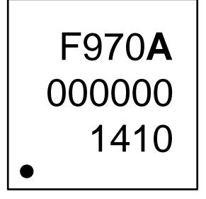
Figure 5.3. QFN-48 Package Marking
