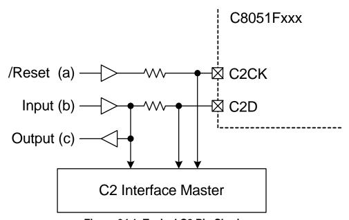
Figure 34.1. Typical C2 Pin Sharing
