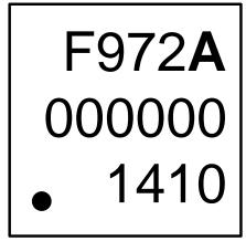
Figure 7.3. QFN-24 Package Marking
