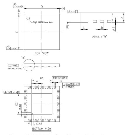
Figure 5.1. QFN-48 Package Drawing (6x6 mm)
