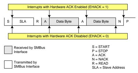
Figure 29.6. Typical Master Read Sequence
