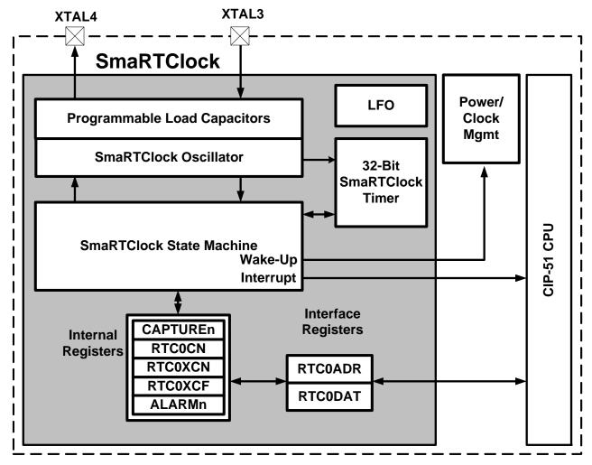
Figure 25.1. SmaRTClock Block Diagram
