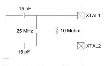
Figure 24.2. 25 MHz External Crystal Example
