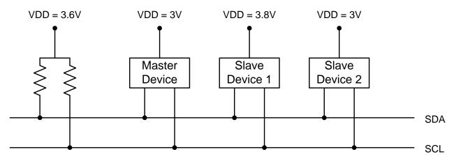
Figure 29.2. Typical SMBus Configuration
