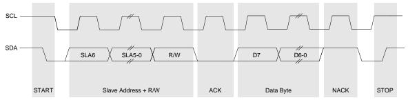
Figure 30.3. I<sup>2</sup>C Transaction
