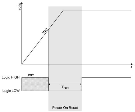
Figure 27.2. Power-on Reset Timing
