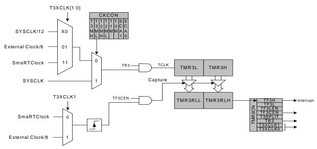
Figure 32.9. Timer 3 Capture Mode Block Diagram
