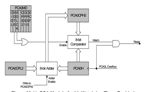
Figure 33.11. PCA Module 2 with Watchdog Timer Enabled
