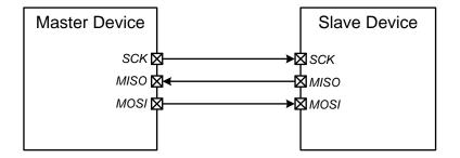
Figure 28.3. 3-Wire Single Master and 3-Wire Single Slave Mode Connection Diagram
