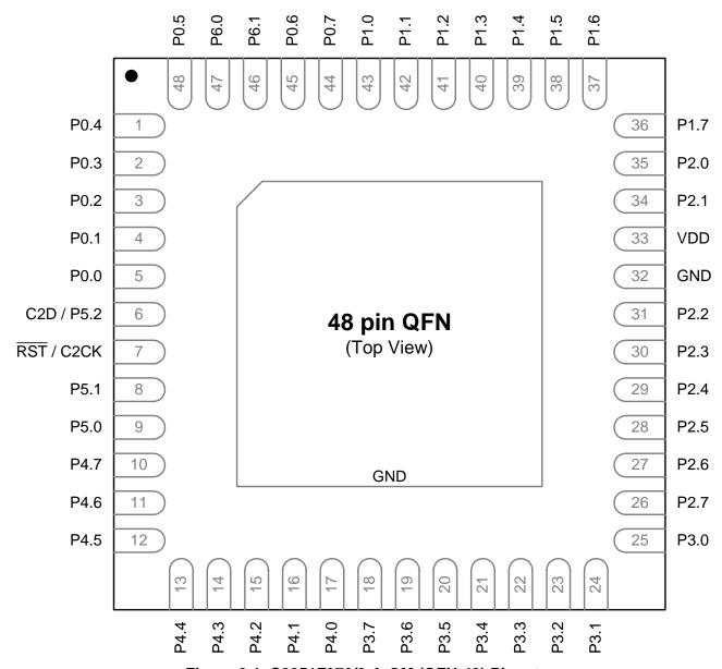
Figure 3.1. C8051F970/3-A-GM (QFN-48) Pinout
