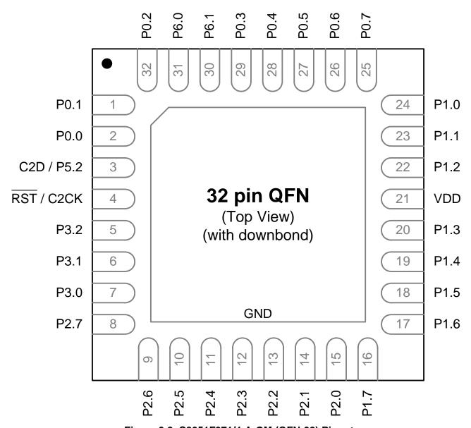
Figure 3.2. C8051F971/4-A-GM (QFN-32) Pinout
