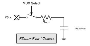
Note: The value of CSAMPLE depends on the PGA Gain. See Table 1.11 for details.
