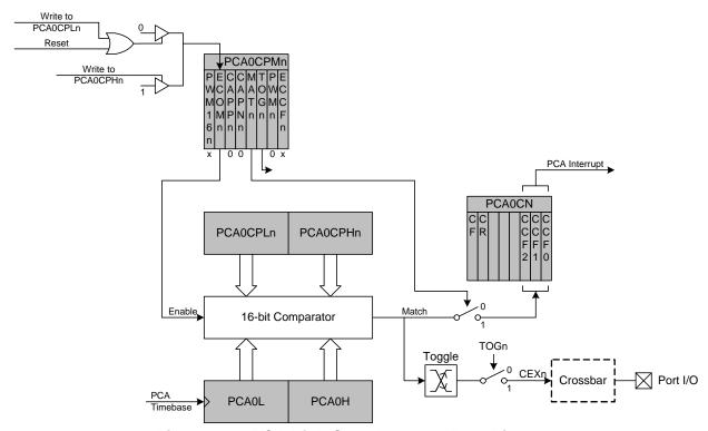
Figure 33.6. PCA High-Speed Output Mode Diagram
