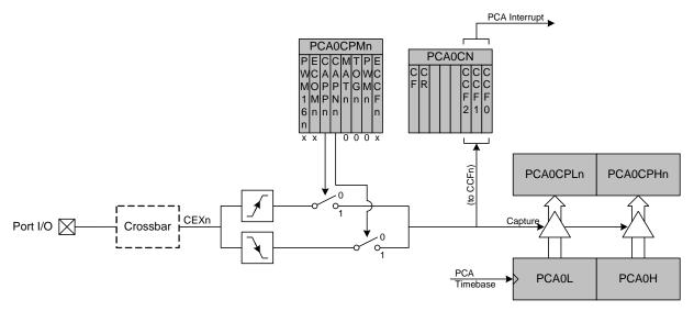
Figure 33.4. PCA Capture Mode Diagram
