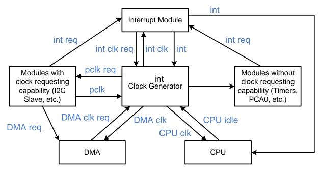
Figure 16.1. C8051F97x Module Clocking in Low Power Modes
