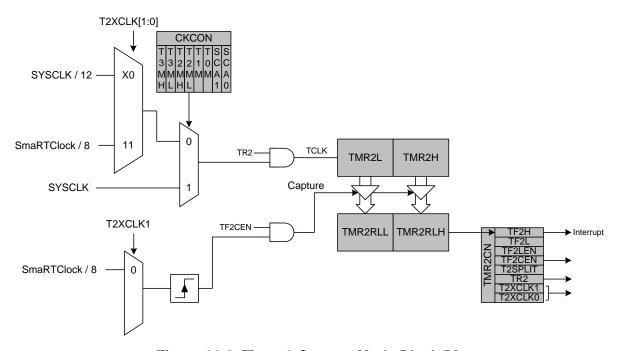
Figure 32.6. Timer 2 Capture Mode Block Diagram
