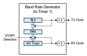
Figure 31.2. UARTO Baud Rate Logic
