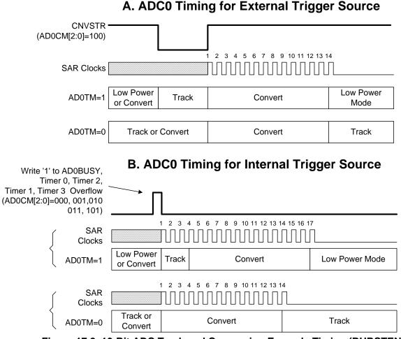
Figure 17.2. 10-Bit ADC Track and Conversion Example Timing (BURSTEN = 0)
