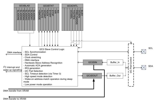
Figure 30.1. I2CSLAVE0 Block Diagram
