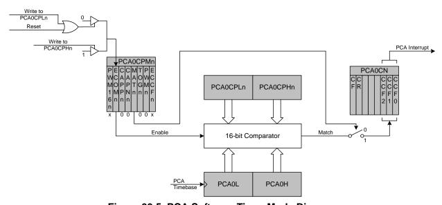
Figure 33.5. PCA Software Timer Mode Diagram
