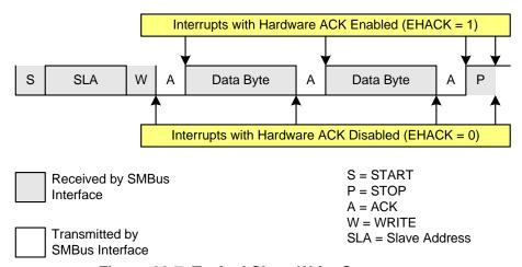
Figure 29.7. Typical Slave Write Sequence
