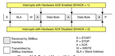
Figure 29.5. Typical Master Write Sequence
