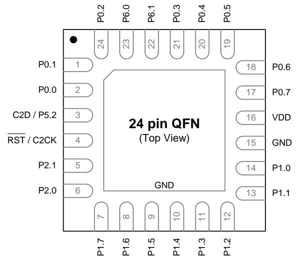
Figure 3.3. C8051F972/5-A-GM (QFN-24) Pinout
