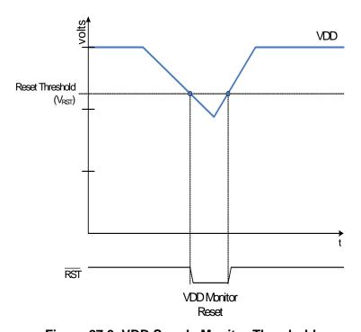
Figure 27.3. VDD Supply Monitor Threshold
