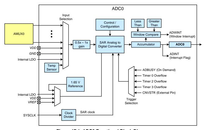
Figure 17.1. ADC0 Functional Block Diagram
