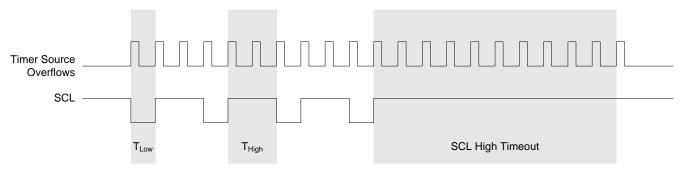
Figure 29.4. Typical SMBus SCL Generation
