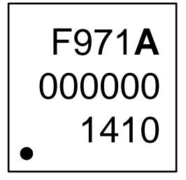
Figure 6.3. QFN-32 Package Marking
