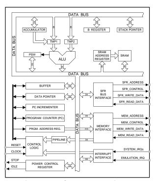
Figure 20.1. CIP-51 Block Diagram
