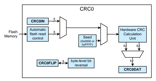
Figure 23.1. CRC0 Block Diagram
