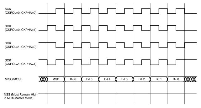
Figure 28.5. Master Mode Data/Clock Timing
