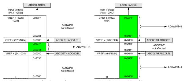
Figure 17.5. ADC Window Compare Example: Right-Justified Single-Ended Data
