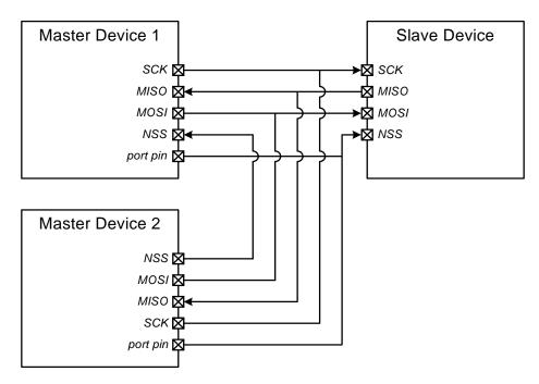
Figure 28.2. Multiple-Master Mode Connection Diagram
