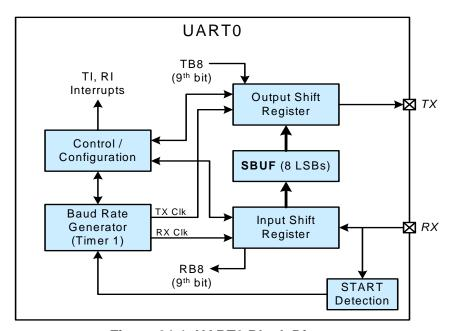
Figure 31.1. UARTO Block Diagram
