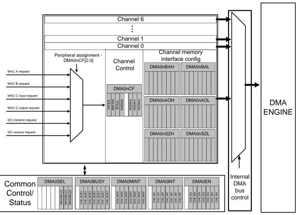
Figure 21.1. DMA0 Block Diagram
