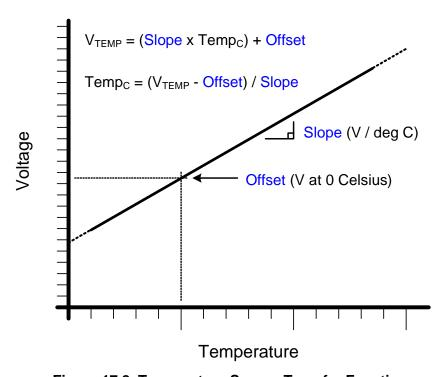
Figure 17.8. Temperature Sensor Transfer Function
