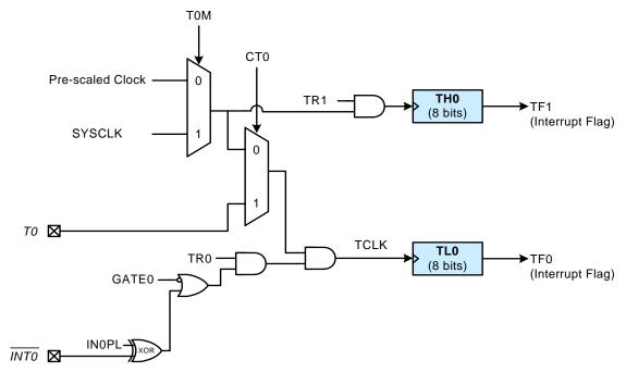
Figure 32.3. T0 Mode 3 Block Diagram
