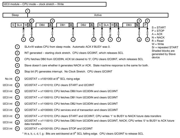
Figure 30.5. Typical I<sup>2</sup>C Write Sequence in CPU Mode
