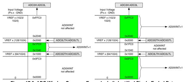
Figure 17.6. ADC Window Compare Example: Left-Justified Single-Ended Data
