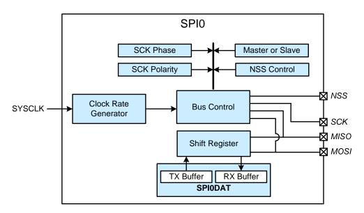
Figure 28.1. SPI0 Block Diagram
