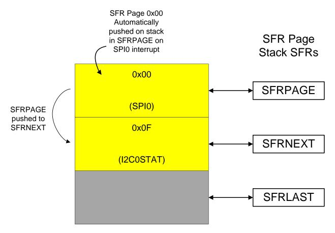
Figure 20.4. SFR Page Stack after SPI0 Interrupt Occurs
