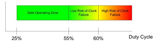
Figure 25.2. Interpreting Oscillation Robustness (Duty Cycle) Test Results
