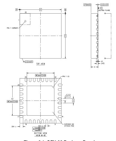
Figure 6.1. QFN-32 Package Drawing
