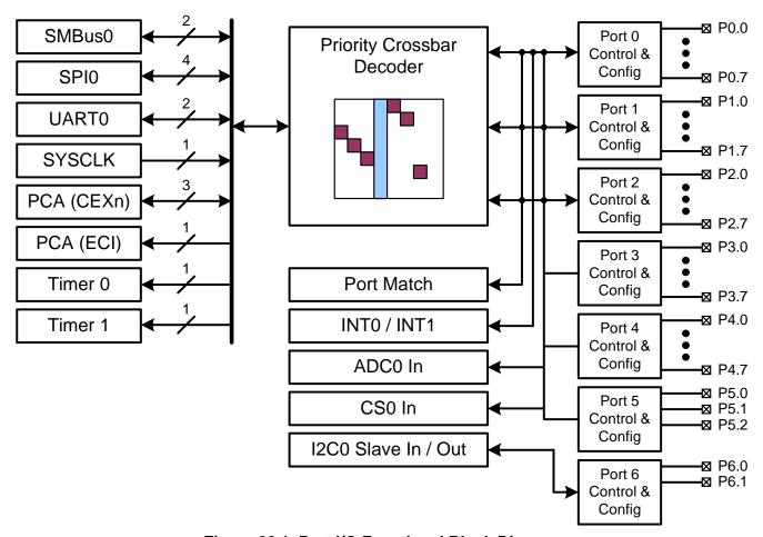
Figure 26.1. Port I/O Functional Block Diagram
