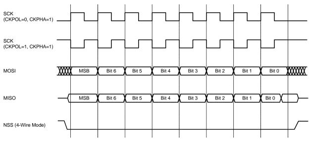
Figure 28.7. Slave Mode Data/Clock Timing (CKPHA = 1)
