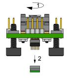
Apply torque and then plug into SF-MLF foot.
