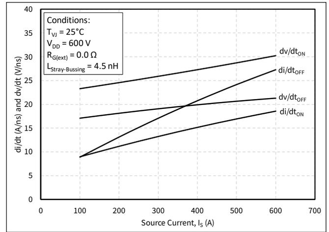
Figure 26.  $dv/dt$  and  $di/dt$  vs. Source Current
