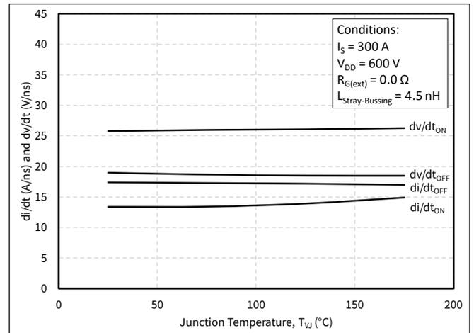
Figure 28.  $dv/dt$  and  $di/dt$  vs. Junction Temperature
