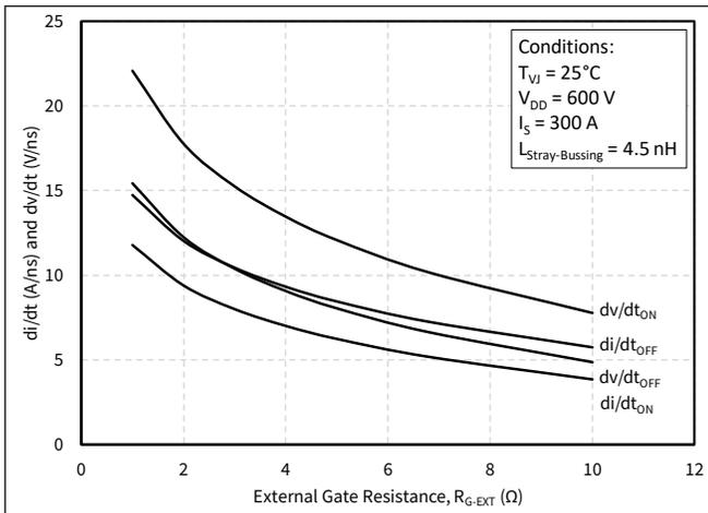
Figure 27.  $dv/dt$  and  $di/dt$  vs. External Gate Resistance
