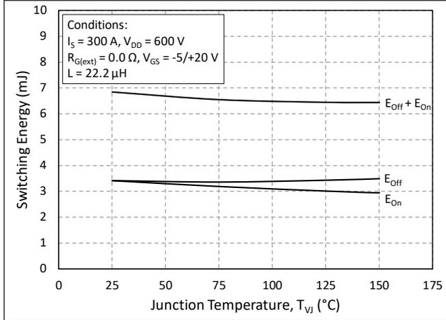
Figure 13. MOSFET Switching Energy vs. Junction Temperature
