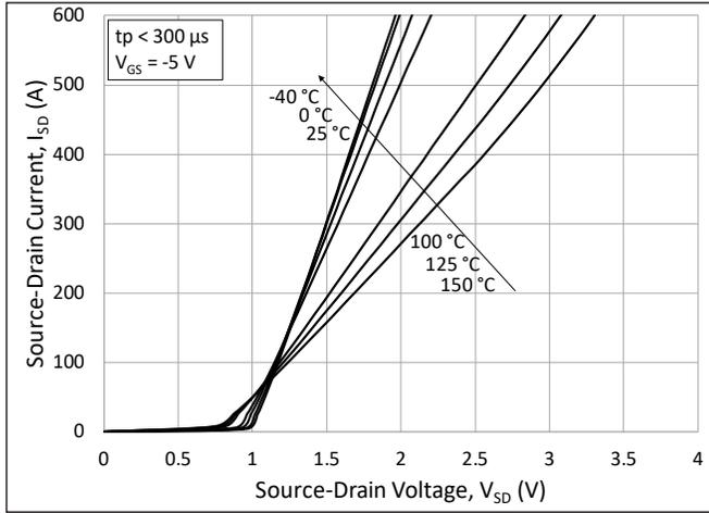
Figure 7. 3<sup>rd</sup> Quadrant Characteristic vs. Junction Temperatures at  $V_{GS} = -4$  V (Diode)
