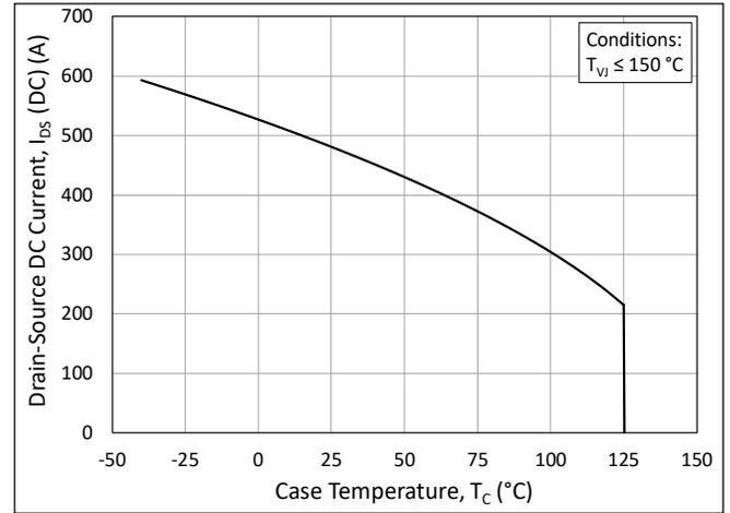
Figure 20. Continuous Drain Current Derating vs. Case Temperature
