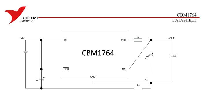
Adj (5 pins): adjustable end. The adjustable output version of the product has this port, and the adj end is directly connected to the reverse input port of the internal operational amplifier. The internal embedded voltage of this port is  $\pm$  7V. The bias current of the port is about 3ua, and the current direction is flowing into the device. The adj terminal voltage is about 1.2V, and the output voltage adjustment range is 1.2V to 20V.
