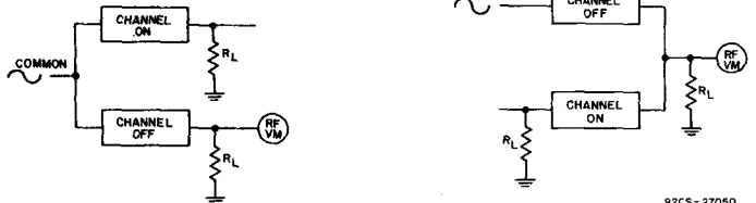
Fig. 25 - Crosstalk between any two channels (all types).
