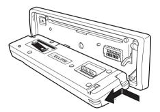
3 Put the front panel into the case.
