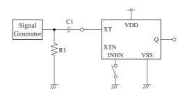
2Vp-p, 10MHz sine wave input signal
