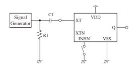
2Vp-p, 10MHz sine wave input signal
