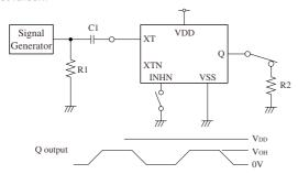
2Vp-p, 10MHz sine wave input signal
