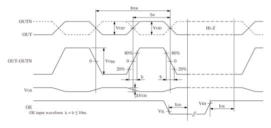
$$\begin{split} \text{DUTY} = 100 \text{t}_{\text{W}} / \text{t}_{\text{PER}} \ (\%) \ @ \ \text{crossing point} \\ \Delta \text{V}_{\text{OD}} = |\text{V}_{\text{OD}} ' - \text{V}_{\text{OD}}| \end{split}$$
