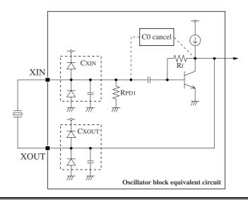
The CF5037 series oscillator circuit has a C0 cancel circuit built-in to improve the oscillator margin. If power is applied when there is an open circuit between XIN and XOUT, self oscillation may occur, which is not abnormal. Users should confirm that the oscillator operates normally when a crystal unit is connected.
