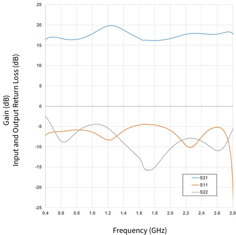
**Figure 3.** Typical Small Signal Response of CGHV40030F-AMP2
