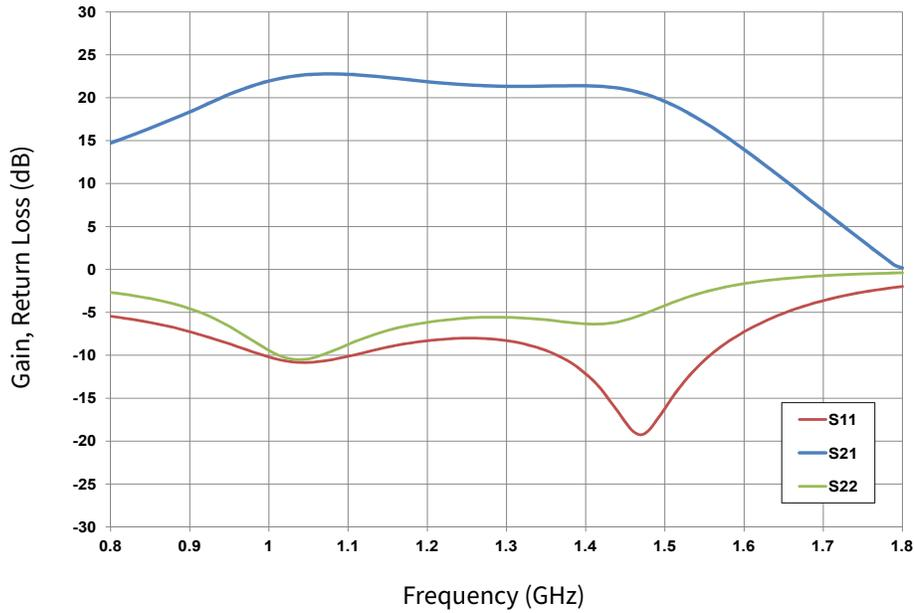
**Figure 1.** Typical Small Signal Response of CGHV40030-AMP Application Circuit
