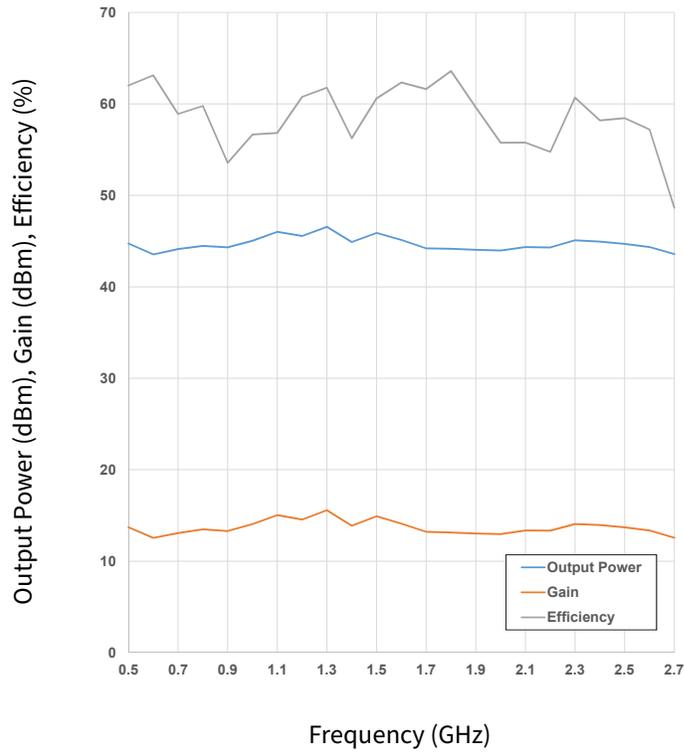
**Figure 4.** Typical Large Signal Response of CGHV40030F-AMP2 Application Circuit
