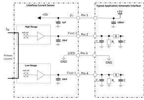
$C_L \ge 1.0$ nF,  $C_L \le 10.0$ nF for EMC protection
