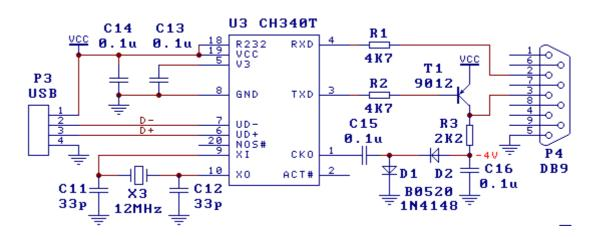
The figure above also shows that USB is converted to RS232. This circuit has the same function as the circuit shown in Section 7.2 except the range of output RS232 is narrower. When R232 pin is driven high, the assistant RS232 function will be enabled, just need to add some diodes, transistors, resistors and capacitors, the special level converter chip U5 in Section 7.2 could be replaced and the hardware cost is lower.
