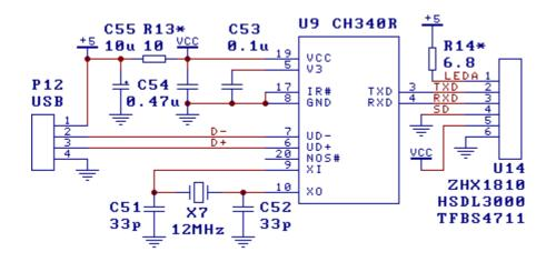
7.6. Connect to MCU and supply power together (figure below)
