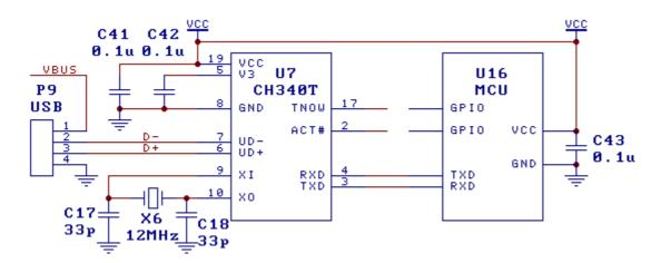
The figure above is a reference design to achieve USB connection on an MCU by connecting it to a CH340 via TTL UART. Here self-power mode is selected, VCC supports 5V or 3.3V (V3 shorted to VCC if VCC is 3.3V), and USB bus power (VBUS) is not used at all (Can be tested by connecting series resistor to I/O of MCU if needed). CH340 shares the same power source with MCU, hence there would be no current inrush
