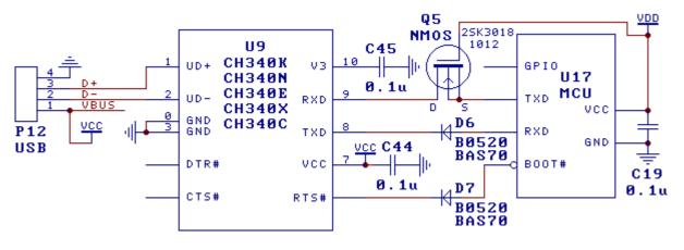
The figure above is a reference design to achieve USB connection on an MCU by connecting it to a CH340 via TTL UART. CH340 is powered by USB bus VBUS. MCU is powered by another power source VDD, VDD supports 5V, 3.3V and even 2.5V, 1.8V.
