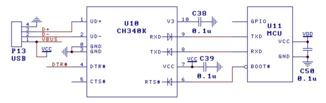
The figure above shows the reference circuit of MCU connecting to CH340K through TTL UART to realize USB communication under dual power supply mode. The CH340K is powered by the USB bus, VBUS (VCC), and the MCU uses another power supply VDD, which supports 5V, 3.3V or even 2.5V and 1.8V. The EPAD of CH340K is an optional GND pin, which can be easily connected to GND or not connected according to PCB routing.
