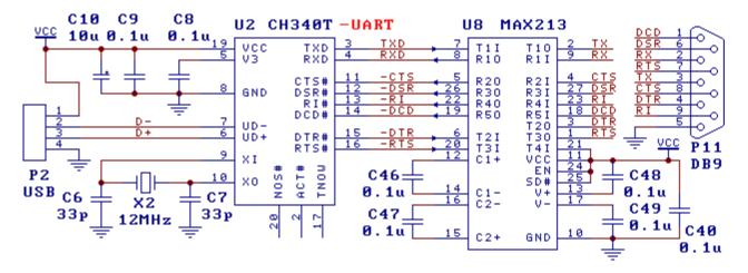
When designing the PCB, pay attention to: C8 and C9 decoupling capacitors must keep close to connection pin of CH340; make sure D+ and D- signal lines are parallel and provide ground or pour copper on both
