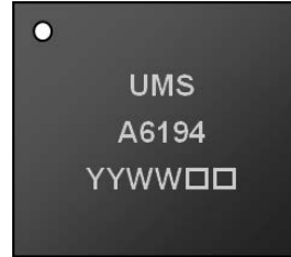
36 lead 6x5 mm QFN package
