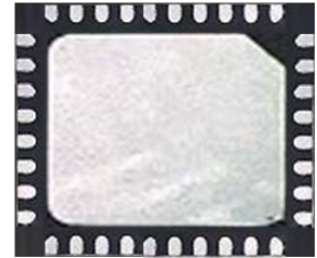
36 lead 6x5 mm QFN package
