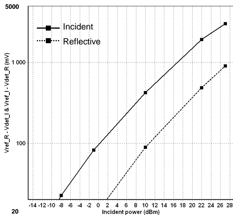
Incident and reflected power detection versus incident power @ 27GHz (Vdetect_I & Vdetect_R)
