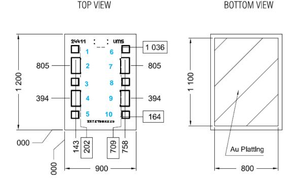
Chip thickness: 100µm +/- 10 µm All dimensions are in micrometers
