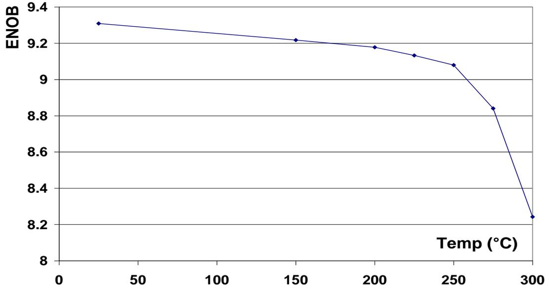
Figure 6: Typical ENOB (=S/(N+D)) over temperature; VDDD=5V
