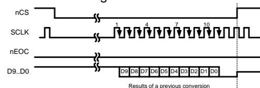
**Figure 16. Reloading the results of a previous conversion.**
