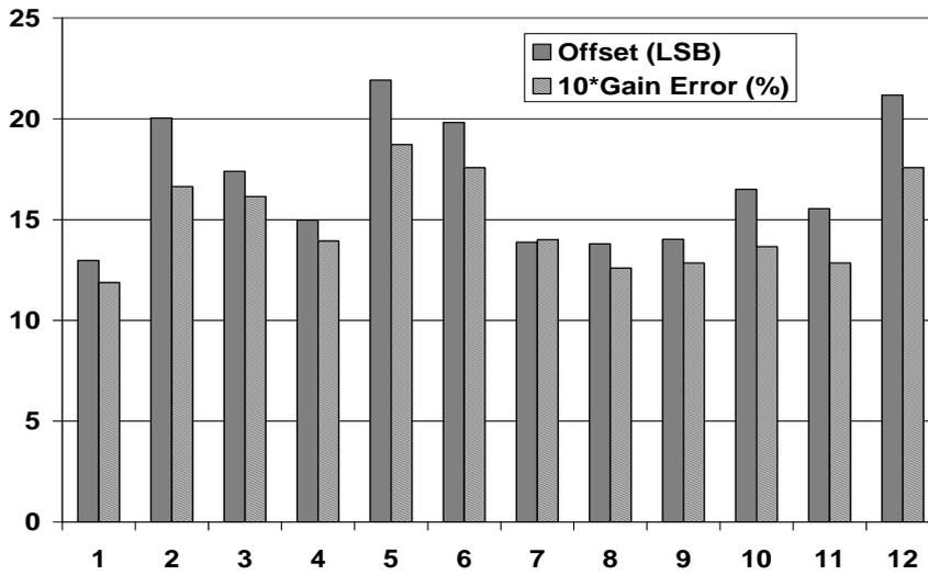
Figure 5: Gain Error (\*10) and Offset (LSB) measured at 25°C on 12 samples from 2 different wafer batches. External CK=200kHz.
