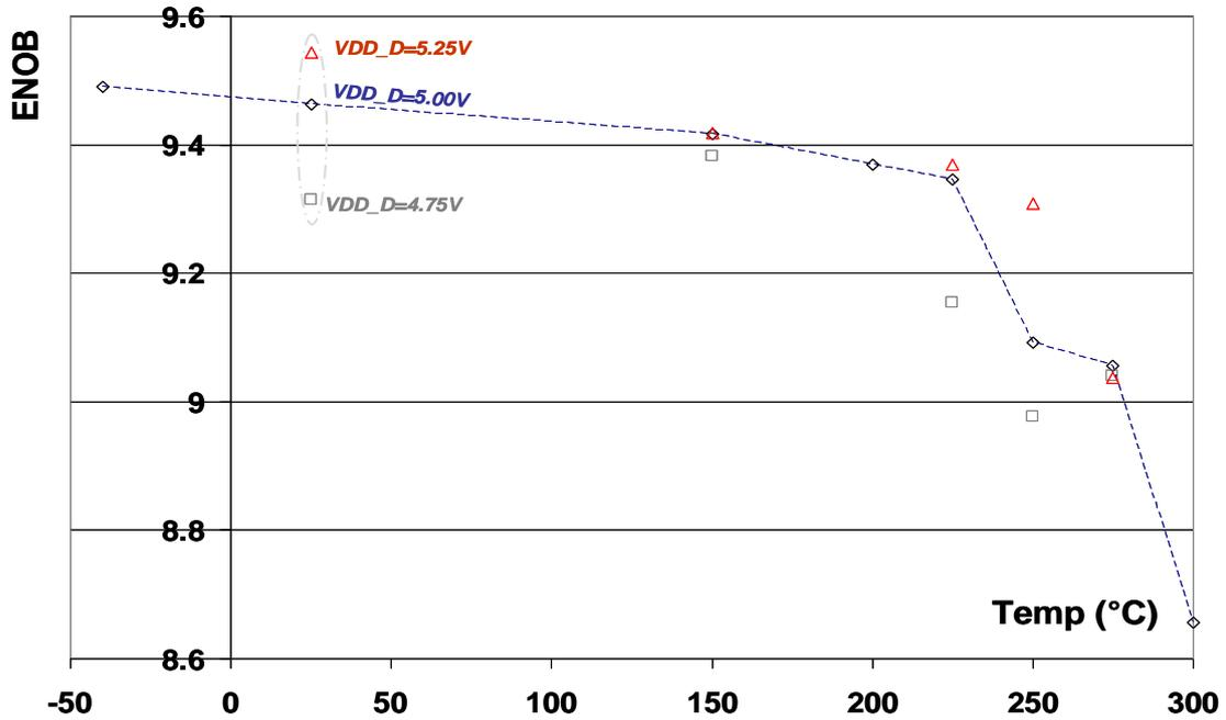
Figure 7: Typical ENOB over temperature; VDDD=4.75V; 5V; 5.25V
