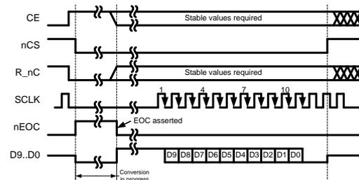
**Figure 15. Conversion cycle and serial read protocol.**
