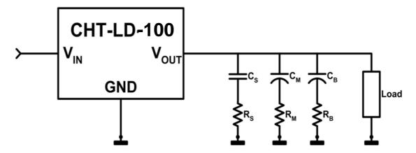
Resistances in series with capacitors represent the internal ESR of these capacitors.
