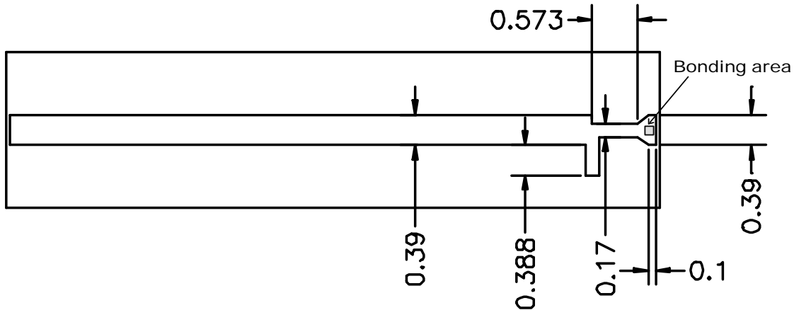
Proposed matching network for a 50Ω transition between OUT1 and a \mu -strip line on DUROID substrate
