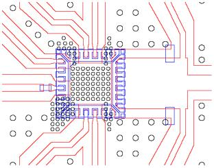
We recommend that all N/C pins be grounded and sufficient number of vias to be present under the ground plane to insure good RF and thermal grounding.
