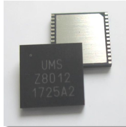
28 leads DFN package-7x7 mm 2
