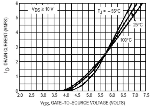
**Figure 2. Transfer Characteristics**
