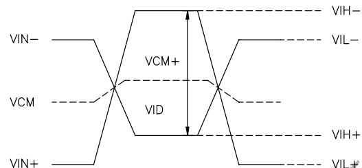
$$\begin{aligned} \text{VID} &= \text{VIN}_+ - \text{VIN}_-, \\ \text{VCM} &= | \text{VCM}_+ - \text{VCM}_- |, \\ \text{VID} &= | \text{VID}_+ - \text{VID}_- |, \\ \text{VID}^+ &= | \text{VIH}_+ - \text{VIH}_- |, \\ \text{VID}^- &= | \text{VIL}_+ - \text{VIL}_- |, \\ \text{VCM} &= (\text{VIN}_+ + \text{VIN}_-)/2, \\ \text{VCM}^+ &= (\text{VIH}_+ + \text{VIH}_-)/2, \\ \text{VCM}^- &= (\text{VIL}_+ + \text{VIL}_-)/2, \end{aligned}$$
