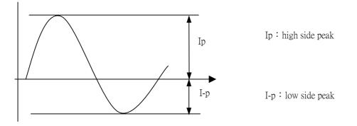
A : The degrees of unbalance =  $| Ip - I-p | / Irms \times 100 (\%)$ B : The ratio of wave height = Ip (or I-p) / Irms
