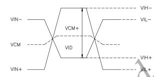
VIN+ : Positive differential DATA & CLK Input VIN- : Negative differential DATA & CLK Input
