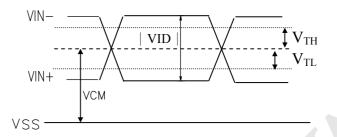
VIN+ : Positive differential DATA & CLK Input VIN- : Negative differential DATA & CLK Input
