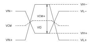
VIN<sub>+</sub>= Positive differential DATA & CLK Input VIN<sub>-</sub> = Negative differential DATA & CLK Input
