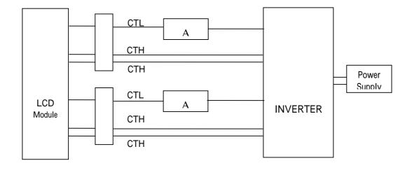
[Note 2] Lamp frequency of inverter may produce interference with horizontal synchronous frequency, and this may cause horizontal beat on the display. Therefore, please adjust lamp frequency, and keep inverter as far from module as possible or use electronic shielding between inverter and module to avoid the interference.
