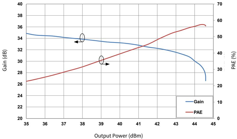
Figure 4. Gain and Power Added Efficiency vs Output Power in the CMPA2735015S
