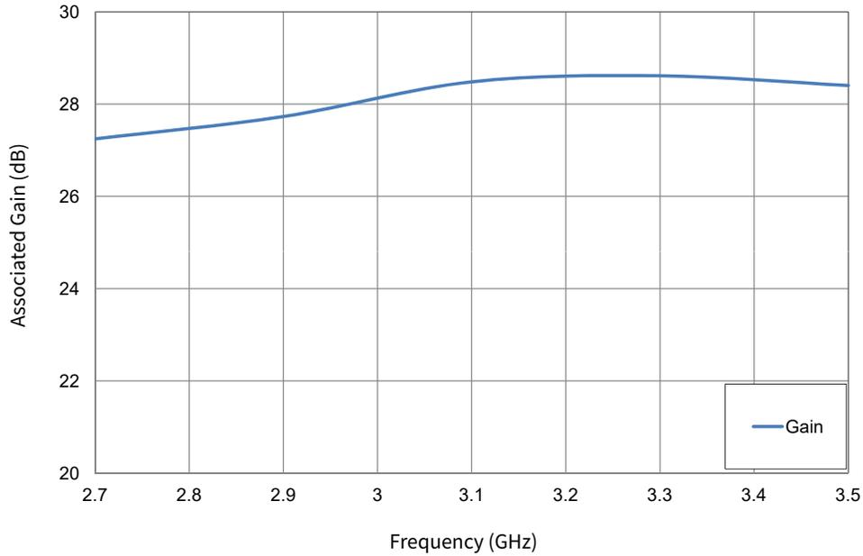
Figure 3. Associated Gain vs Frequency in the CMPA2735015S
