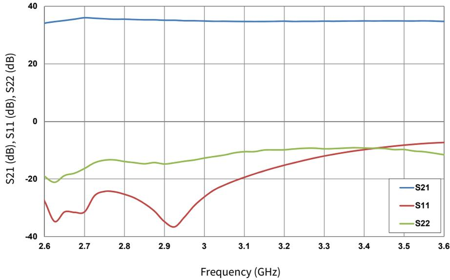
Figure 1. Gain and Input Return Loss vs Frequency in the CMPA2735015S
