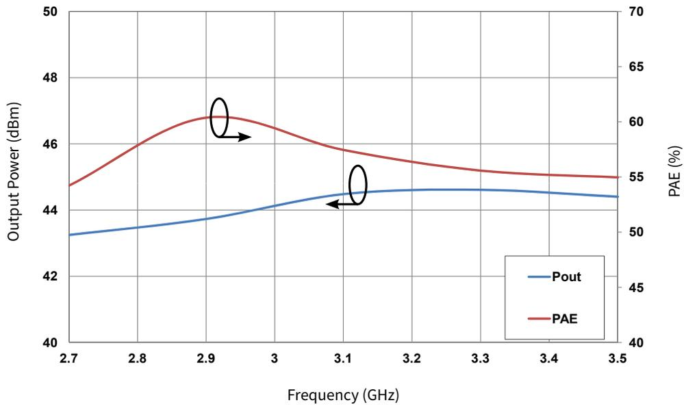
Figure 2. Output Power and PAE vs Frequency in the CMPA2735015S
