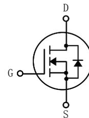
N-Channel Enhancement Mode Field Effect Transistor
