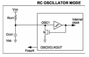
The oscillator frequency, when in EXT RC, divided by 4, is available on the OSCOUT/P0.6 pin, and can be used for test purposes
