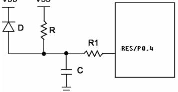
External Power-On Reset circuit is required only if VDD power-up is too slow. The diode D helps discharge the capacitor quickly when VDD powers down.
