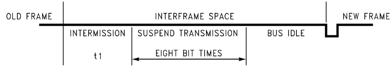
FIGURE 23. Interframe Space for Nodes Which Are Error Passive and Have Been Transmitter for the Last Frame
