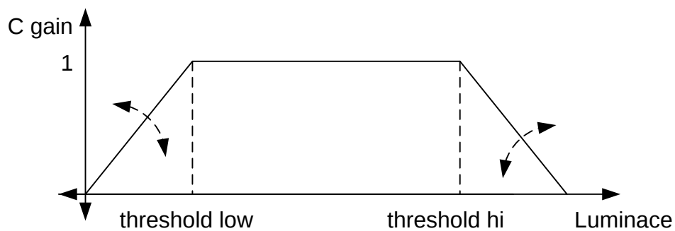
Figure 10-16 Applying Gain on Luminance Threshold
