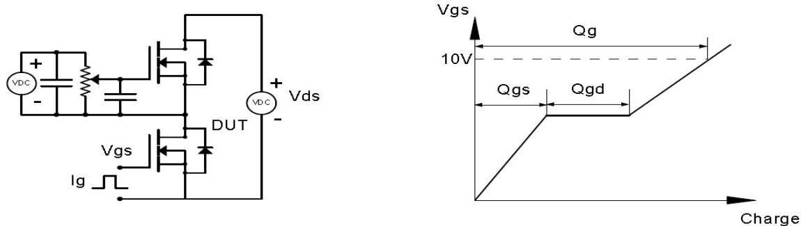
Resistive Switching Test Circuit &amp; Waveforms
