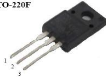
1. Gate 2. Drain 3. Source
