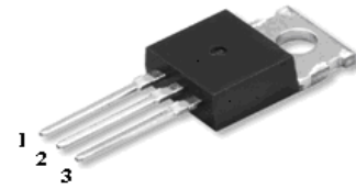
1. Gate 2. Drain 3. Source
