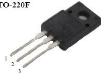
1. Gate 2. Drain 3. Source
