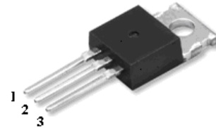
1. Gate 2. Drain 3. Source
