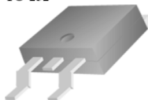
1.Gate 2.Drain 3.Source
