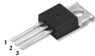
1. Gate 2. Drain 3. Source
