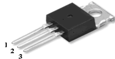
1.Gate 2. Drain 3. Source
