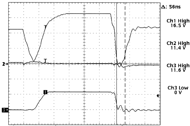
Channel 1 – GATE(H) (5.0 V/div) Channel 2 – GATE(L) (5.0 V/div) Channel 3 – Inductor Switching Node (10 V/div)
