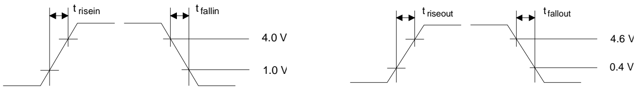
Figure 1. Rise and Fall Times
