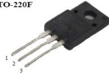
1. Gate 2. Drain 3. Source
